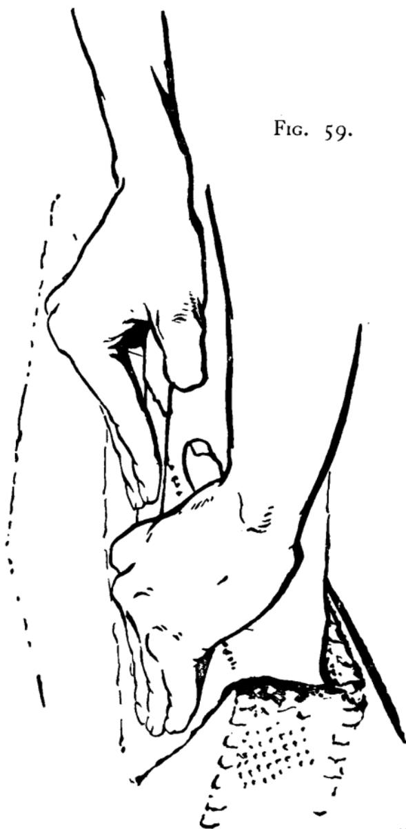
on the under side. This burr is got by rubbing the knife on the lithographic stone on which the paring is done. The handle of the knife should never be raised to such a height above the surface of the stone that it is possible to get the under fingers of the right hand over the edge of the
