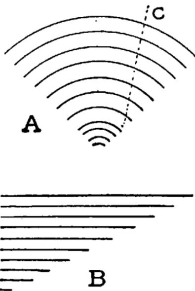
centric circles (see fig. 80, A). The portion of the curves cut off by the dotted line C will make a second set with flatter curves. Gouges are used for tooling curved lines.
