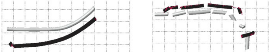
Fig. 7.44 Comparing simulations results ( grey ) with experiments ( black ) of yawed impacts, for plates moving towards the rod ( left ) and away from it ( right )
