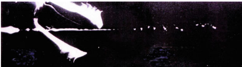
Fig. 7.45 Jet disruption by a reactive cassette
